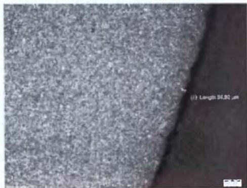
Fig. 10. Depth of decarburized layer on rolled section steel in coils with diameter 16.5 mm according to GOST 1763 (experimental cooling mode)
