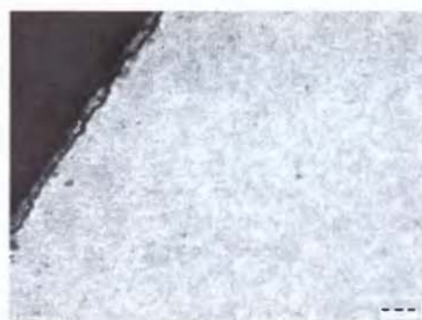
Fig. 14. Depth of decarburized layer on rolled section steel in coils with diameter 16.5 mm according to GOST 1763 after spheroidizing annealing (experimental cooling mode)
